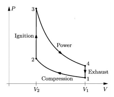
Start by determining the work and heat associated with each of the four processes connecting points  $1 \to 2 \to 3 \to 4 \to 1$ :
