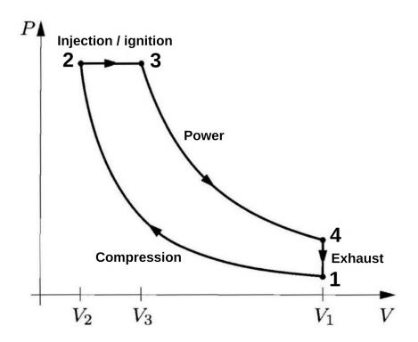
(a) By computing  $W_{out}$ ,  $W_{in}$  and  $Q_{in}$ , show that the Diesel cycle's efficiency is
