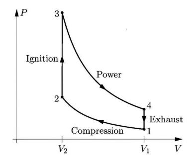
The efficiency  $\eta$  of the Otto cycle depends on the **compression ratio**
