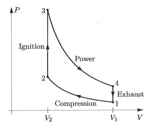
The efficiency  $\eta$  of the Otto cycle depends on the **compression ratio**
