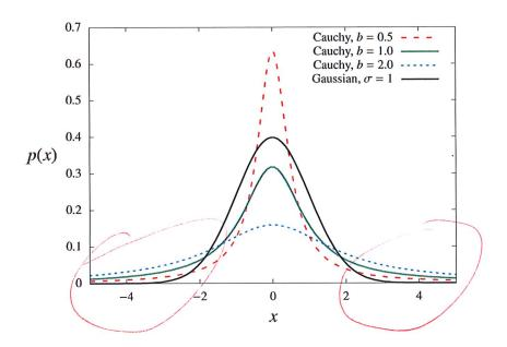
The figure shows how the peak of the Cauchy–Lorentz distribution around x=0 becomes higher and narrower as b decreases. Even when its peak is very narrow, as |x| increases  $p_C(x)$  again becomes larger than the gaussian distribution, simply because the latter decreases exponentially quickly while  $p_C(x)$  decreases only  $\sim 1/x^2$ . These "fat tails" at large |x| make the Cauchy–Lorentz distribution both interesting and challenging to analyze.
