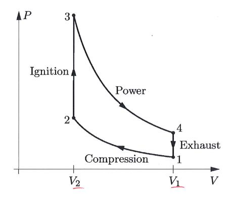
The efficiency  $\eta$  of the Otto cycle depends *only* on the compression ratio r. What is this efficiency? How does it compare to the efficiency of the Carnot cycle? How should  $V_1$  and  $V_2$  be chosen to maximize the efficiency?
