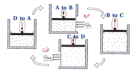
The illustration above supposes that the hot reservoir is located to the right of the system, while the cold reservoir is located to its left. In words, the four stages are the following:
