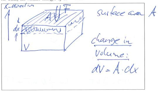
Since we move the piston against the force F > 0 from the pressure in the container, our energy changes by the amount dE (which would be smaller than zero in the present setting):
