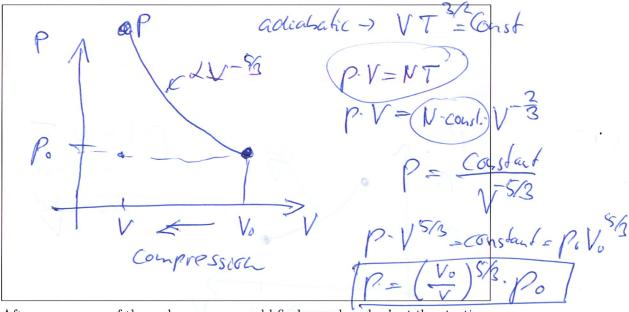
After a sequence of these changes, we could find ourselves back at the starting point in the p-V-diagramme. We call the whole process a thermodynamic cycle, since we could repeat the process over an over again. As we will see below, thermodynamical cycle can take heat from a hot reservoirs to a cold reservoir and convert part of it into work. This is e.g. used in car engines, refrigerators or heat pumps.
